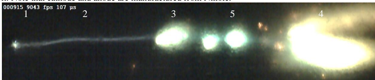
FIGURE 1. Heterogeneous plasmoids (3) created by pulsed- repetitive electrical discharge (2) in the experimental setup PVR. Cathode-injector (4) - right, anode (1) - left. Erosive metal micro droplets-5
