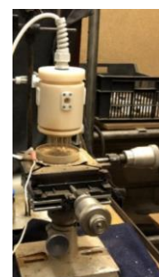
FIGURE 1. a. Schematic diagram of the experiment with a corona discharge above the surface of a liquid: 1 - dielectric cell. 2 - liquid. 3 - copper anode. 4 - rack. 5 - copper cathode. 6 - power source. b. The device of a multi-needle corona (19 needles).
